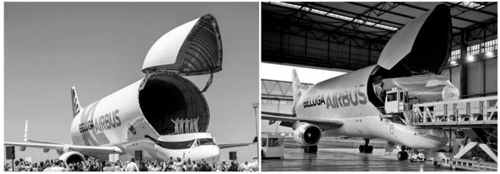
Beluga XL has 30% more payload capacity than Beluga ST, which is based on Airbus A300-600 passenger aircraft. With the ability to accommodate a pair of A350 XWB aircraft wings, the new-generation aircraft will address the transport capacity needs for the ramp-up of A350 XWB.
