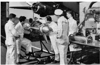
In 1945 United installed Sperry Electronic Automatic Pilots in the "230" (DC-4) planes replacing Hydraulic Automatic Pilots used in the past.
