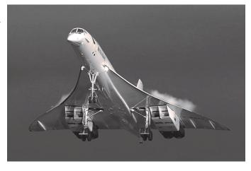
Dry thrust: 32,000 lbf each. Thrust with afterburner: 38,050 lbf each. (Not really a whole lot! 8)
