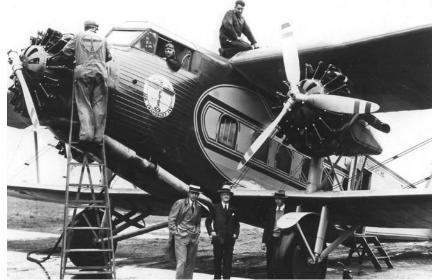
and leather upholstered seats. Powered by three 425 hp Pratt & Whitney "Wasp" engines, it had a cruising speed of 115 mph with a range of 545 miles and a service ceiling of 14,000 ft. The gross weight was 15,276 pounds.
